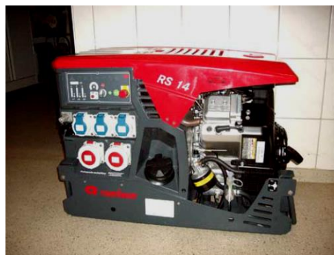
14 KVA Notstrom Aggregat
